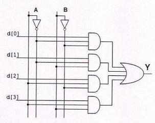
➤ Thus Data input can be selected from any one of 4 – input lines D<sub>0</sub>,D<sub>1</sub>,D<sub>2</sub> and D<sub>3</sub> this multiplexer circuit is also termed as Data Selector.
