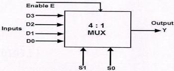
The logic expression for the 4:1 multiplexer output can be derived in terms of data input and data select/control input and is given as:
