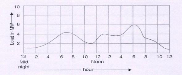
**Load curve:** The curve showing the variation of load on the power station with respect to time is known as load curve.
