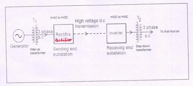
The following are the main components of HVDC transmission system:
